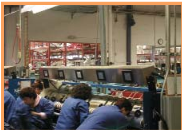
With multiple display units, employees see real-time efficiency information. The Greer Monitoring System provides information not only for individual items but also daily shift totals.
