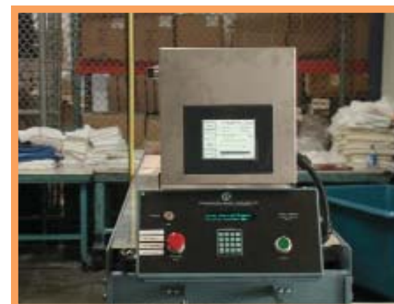
With Ethernet-based controllers, employees can switch to different stations and still monitor daily efficiency with the Greer Monitoring System.
